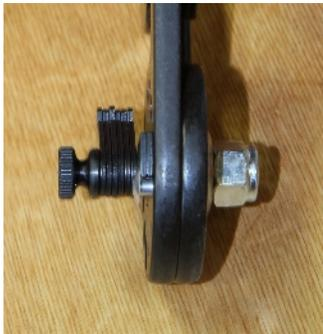
*Cutting rivet to length using two 1/16" thick spacers + 1/4" thickness of cutter = 6/16" or 3/8" length*
