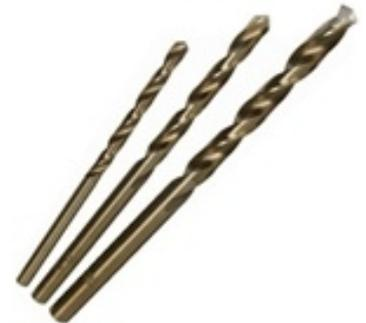
Drill bits sold by Vintage Trailer Supply have a split tip, which means that each flute or starting face is ground in such a way that there are two points of contact with the metal. This feature helps keep the bit centered
