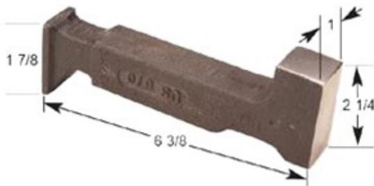
A **bucking bar** is a hand-held anvil as stated in the Basic Principles section. The bucking bar sold by VTS has three faces that can properly reach almost any rivet tail location encountered in bucking rivets in a recreational vehicle. It is important to keep the faces of the bucking bar clean and corrosion free. To store this tool, spray a little corrosion preventive to keep it in good shape for the future.
