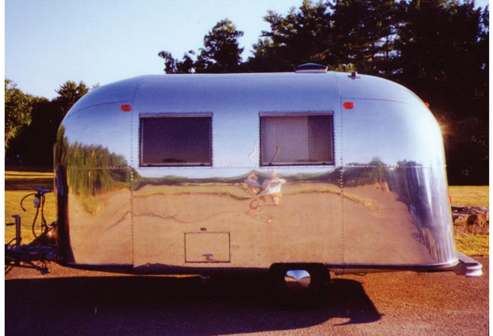
the trailer skin its strength. The pure aluminum cladding is soft and is what shines up so well when polished.
